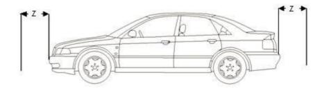
Dimension Z = 100mm which is the maximum longitudinal extent permissible forward or rearward projection from the bodywork. (MSAJ5.2.7)
